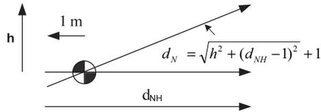
Figure 2-8 Distance measured to top of primary barrier.
